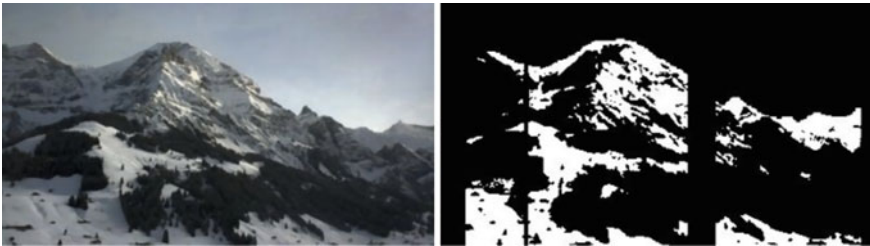
Fig. 7.7 Example of an image and of the snow mask generated from it
