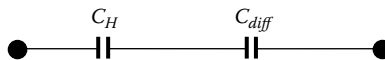
FIGURE 2.5 Helmholtz and diffuse layer differential capacitances ( C_H and C_{diff} respectively) connected in series.
