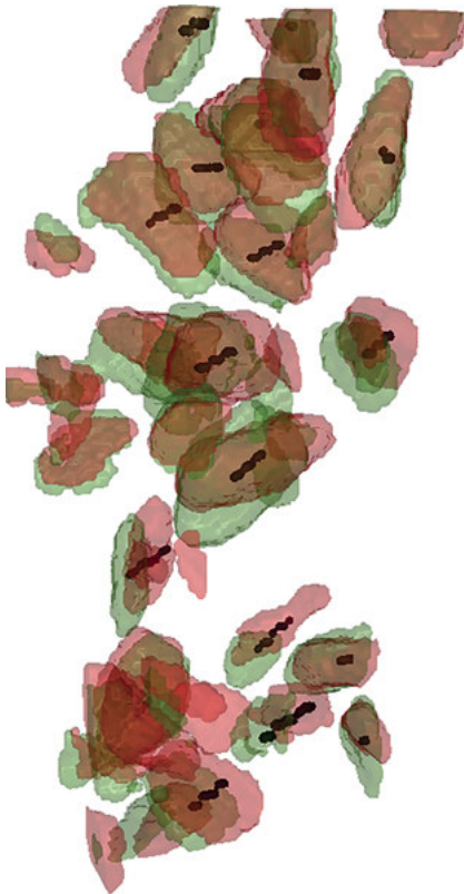
Figure 17.7: Here, the assigned particles without (green) and with a 240 mT field (red) are shown. The black lines represent the trajectory of the assigned particles. A rotation of the particles is visible as well. [23]
