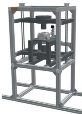
(b) CAD drawing of coil assembly
