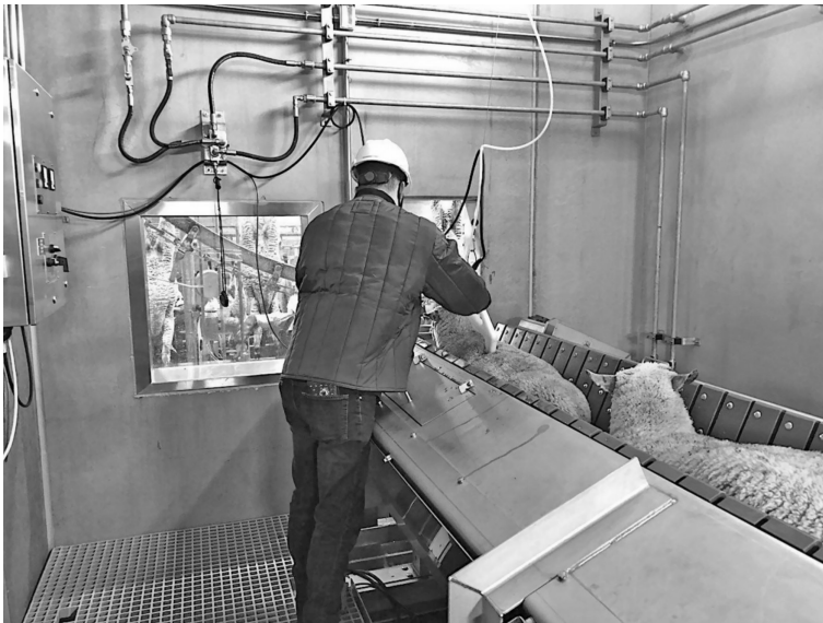
Figure 12.6 Head to back electrical stunner being used on sheep. This device simultaneously passes the electric current through the brain and the heart to produce both instantaneous unconsciousness and cardiac arrest. The sheep are riding to the stunning a V-conveyor restrainer (photo credit: Temple Grandin).
