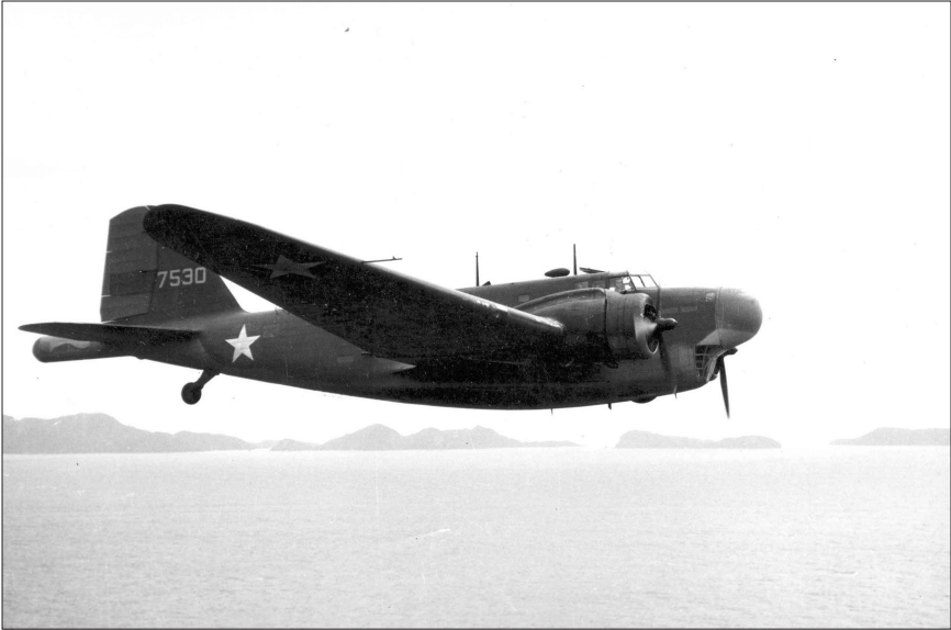
Douglas B-18B (S/N 37-530, originally a B-18A) with the Magnetic Anomaly Detection (MAD) tail boom. B-18s were frequently used for anti-submarine warfare in the Caribbean theatre (U.S. Air Force Photo). Source: National Museum of the US Air Force, http://www.nationalmuseum.af.mil .
