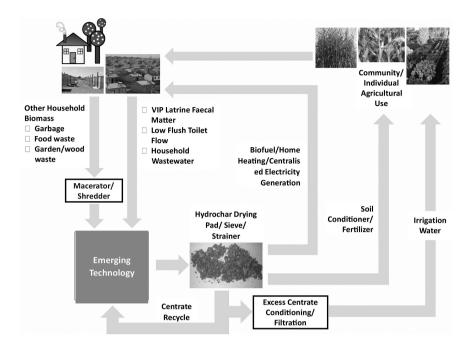
**FIGURE 3.6** Detailed schematic illustration for application of the EHTP processing faecal sludge from low-cost sanitation systems at a centralised facility in combination with another household biomass.
