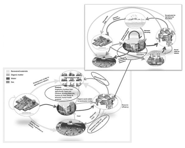
**FIGURE 3.9** Illustration of potential coupling of EHTP process with other technologies within the material pathway (Adapted from IWA, 2016 and Musvoto & Mgwenya, 2022).
