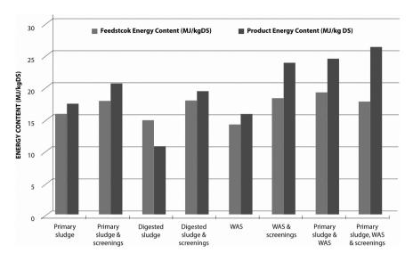
**FIGURE 3.3** Energy content values for different feedstock combinations processed by the EHTP process and generated products (hydrochar).
