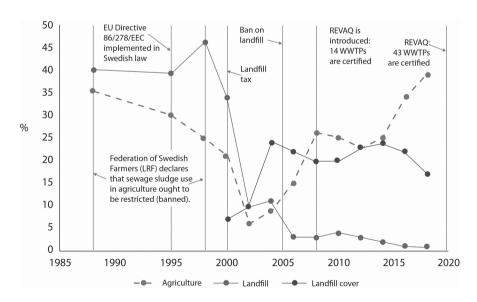
**FIGURE 2.1** The use of sewage sludge in Sweden, 1988–2018 (percentage shares).
