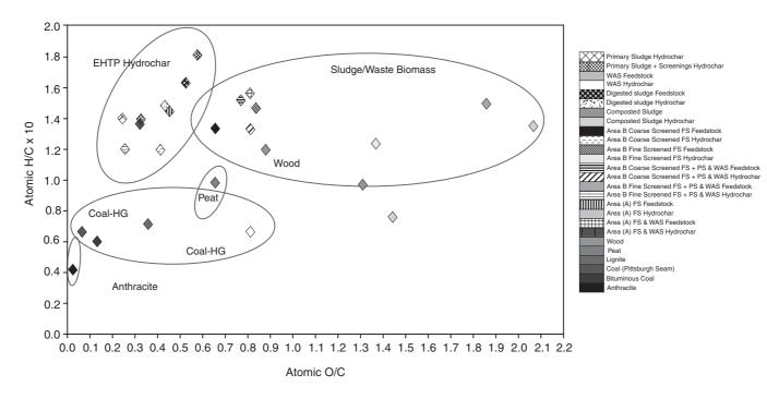
FIGURE 3.4 Van Krevelen diagram for sludge feedstocks, hydrochars from the EHTP process, coals and other fuels.
