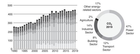
**FIGURE 13.1** Incremental  $CO_2$  emissions by sector from 1990 to 2019 in South Africa from fuel combustion (MtCO<sub>2</sub>/year). Power generation remains the main  $CO_2$  contributing sector.
