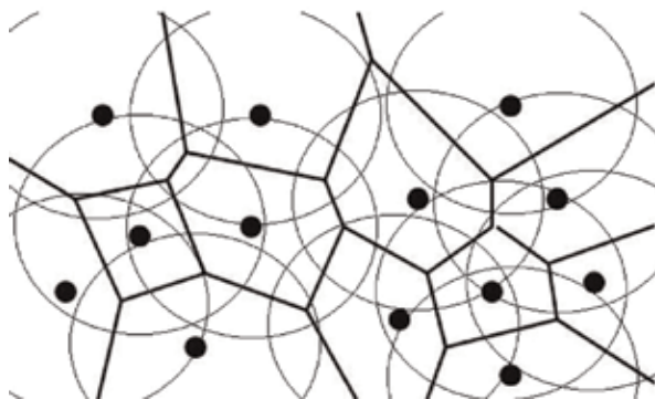
Figure 2. Example of subdivision of the x, y plane in Voronoi cells.
