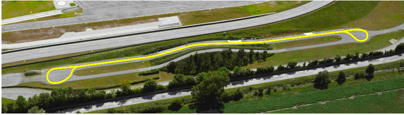
Figure 4.7: Test track and path used for learning experiment with disturbances (modified from [49]). During learning, the vehicle was repeatedly driven over a hill with slopes of 12% and 16% and turned after passing over it. After each pass the vehicle was turned with maximum steering angle to stay within the paved area. Tight turns and slopes act as disturbances on longitudinal dynamics. Since these disturbances affect the vehicle only briefly, the steady-state compensation in the low-level controller can only partly compensate them. The path repeatedly driven during experiments is marked in yellow.
