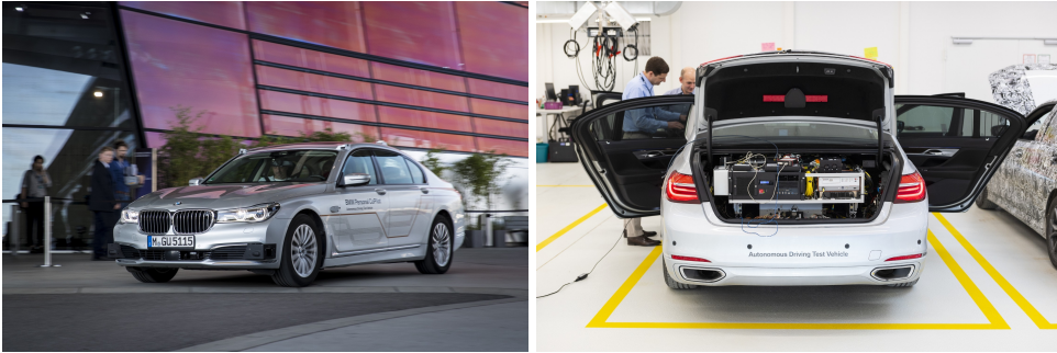
Figure 4.4: Test vehicle based on a BMW 740Li [17, 18] used for online training. It is equipped with a dSpace Autobox that runs our proposed algorithm online, closed-loop and in real time. It accesses controllers for chassis/brake and powertrain via in-vehicle bus systems.
