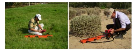
Plate 1.6 EC measurement with EM 38 in vertical mode (left: grassland) and horizontal mode (right: *Atriplex* field)
