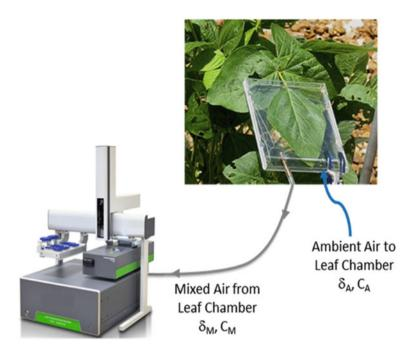
Fig. 6.10 Experimental setup for measuring  $\delta_M$  and  $C_M$
