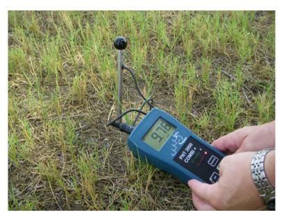
Plate 1.5 Salinity monitoring in a grass field using salinity probe. (Field scout PNT 3000 COMBI+)
