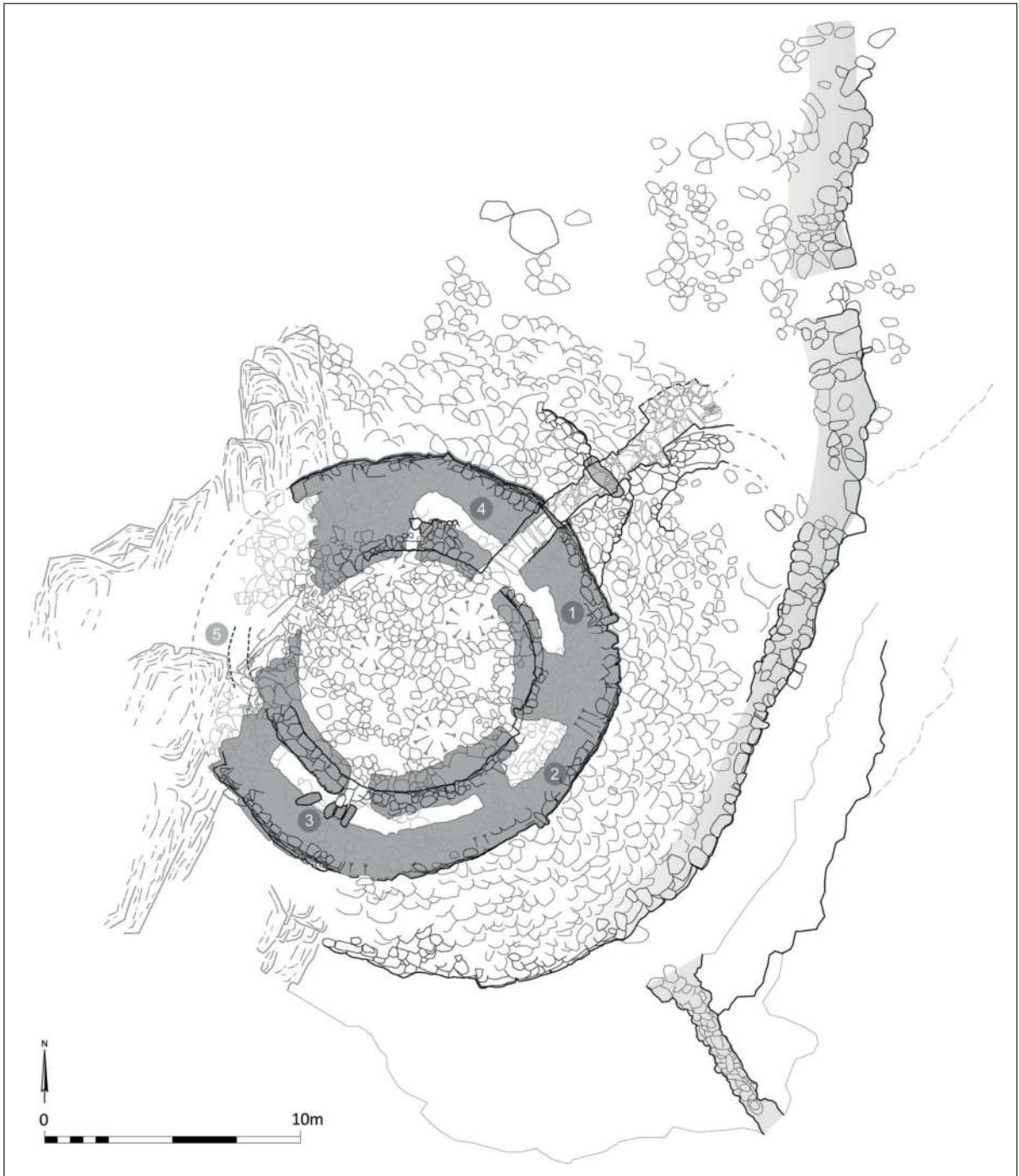
Figure 2A.2 Plan of the broch at wall head level, with the ground level footprint shown as shaded grey. The cell numbers are indicated
