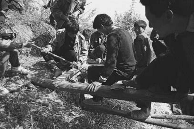
FIG. 6. Turning a bowl on the pit-lathe
