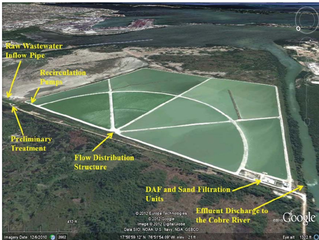
Figure 1.120 The Soapberry wastewater treatment plant in Kingston, Jamaica, based on a lagoons system followed by DAF followed by sand filtration
