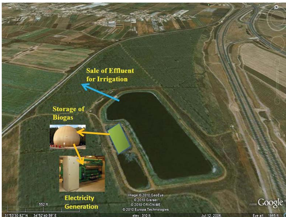
Figure 1.124 Recovery of resource from wastewater in the naan wastewater treatment and stabilization reservoir system
