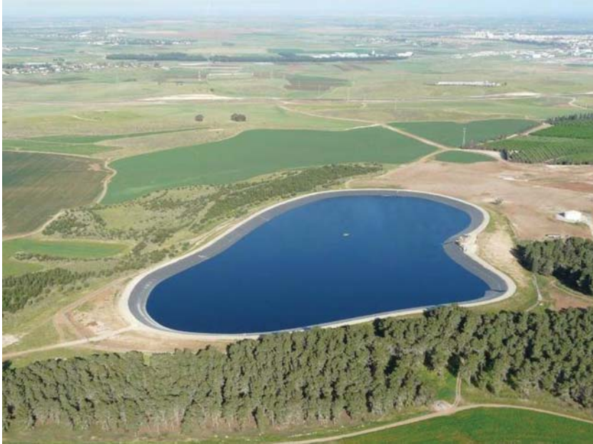
Figure 1.24 A typical reservoir almost filled with effluent towards the beginning of the irrigation season
