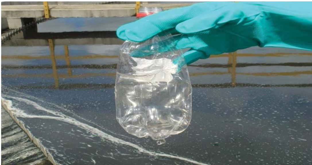
Figure 1.67 The effluent of the Tibagi treatment plant, Parana, Brazil (Effluent Quality: BOD 5–25 mg/l, COD 40–100 mg/l, TSS 4–10 mg/l)
