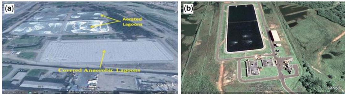
Figure 1.116 (a) Carapongo Treatment Plant near Lima, Peru, based on Covered Anaerobic Lagoons followed by Aerated Lagoon; (b) The Fazenda Rio Grande Treatment Plant in Parana, Brazil, based on UASB followed by an Aerated Lagoon followed by a Facultative Lagoon
