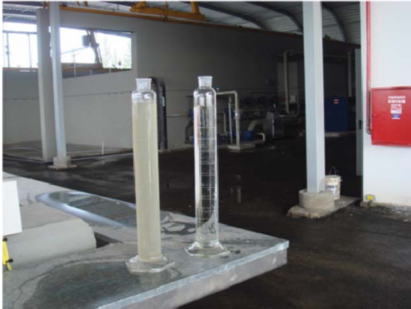
Figure 10.25 Samples of effluent and raw sewage of the ben gurion MBR treatment plant
