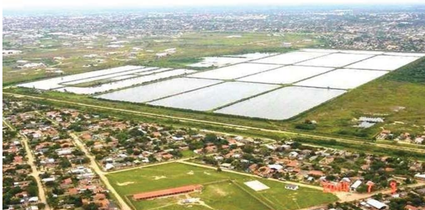
Figure 1.12 Air photo of a conventional anaerobic-facultative-maturation lagoons plant for municipal wastewater treatment, Plant E, one of three in the City of Santa Cruz, Bolivia
