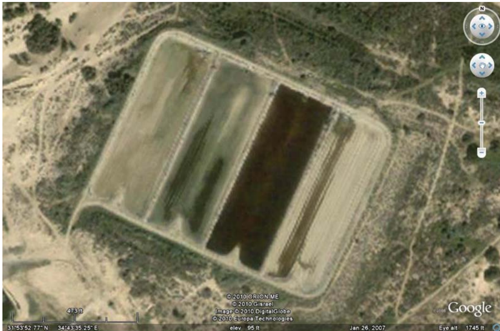
Figure 1.44 Satellite photo of one of the effluent infiltration basins of the Dan Region wastewater reuse project in Israel, serving the metropolitan area of Tel Aviv
