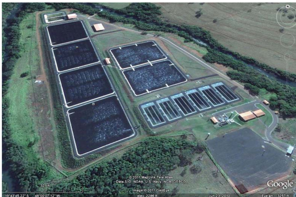
Figure 1.81 The treatment plant of Uberaba consisting of UASB followed by aerated lagoons
