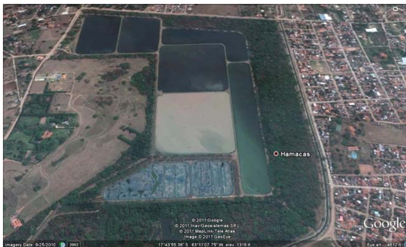
Figure 1.53 A satellite photo of the upgraded N2 lagoons plant in Santa Cruz, Bolivia
