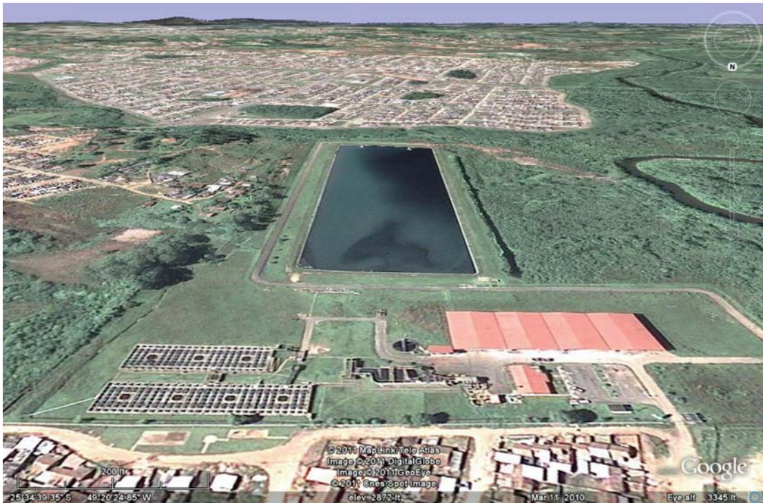
Figure 1.63 The Padilha Sul Plant in Curitiba, Parana, Brazil, based on UASB followed by facultative lagoons
