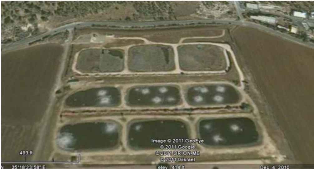
Figure 1.82 The pre-treatment unit of the wastewater treatment plant of Nazareth consisting of anaerobic lagoons followed by aerated lagoons
