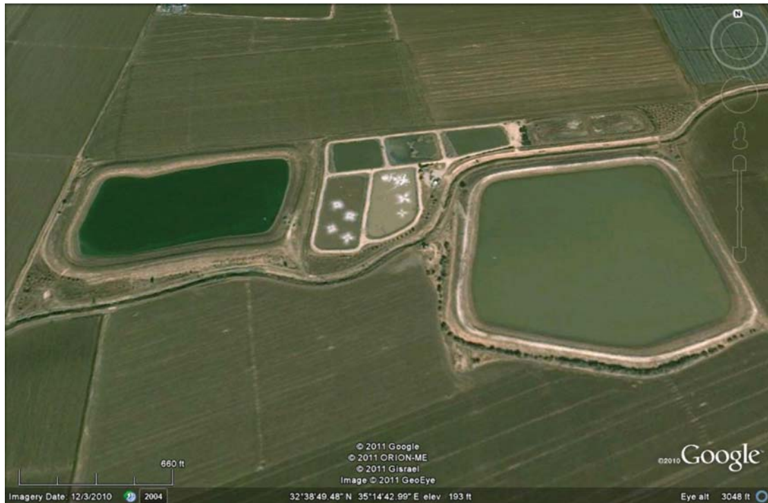
Figure 7.7 A stabilization reservoirs system consisting of pretreatment by anaerobic lagoons followed by aerated lagoons and two reservoirs which can be operated as a sequential batch system
