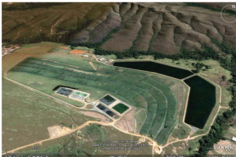
Figure 1.91 Satellite photo of the sao sebastiao treatment plant in Brasilia, Brazil, consisting of UASB followed by overland flow followed by lagoons
