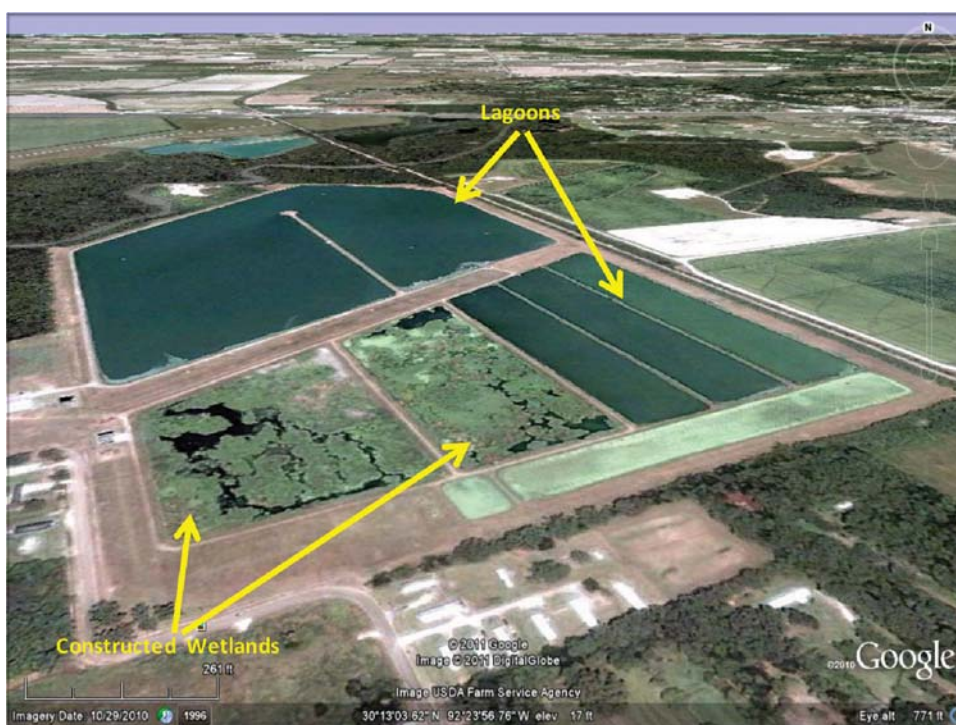
Figure 1.112 The treatment plant of Crowley, Louisiana, based on facultative lagoons followed by constructed wetlands
