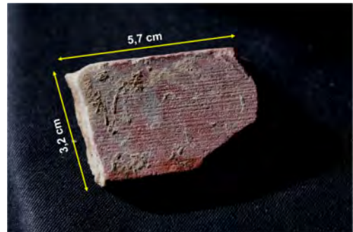
Figure 2. View of the back of a small decorative cornice. The surface is completely covered with traces of sawing, slightly marked and very close to each other.
