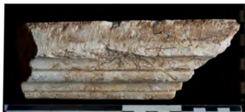
Figure 7. Decorative cornice fragment with flat chisel marks on one of its surfaces. This surface was not visible when the piece occupied its original place in the building's decorative program.
