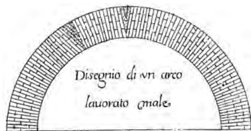
Figure 4. Example of a “badly built” brick arch (Balducci 1682: unnumbered plate).
