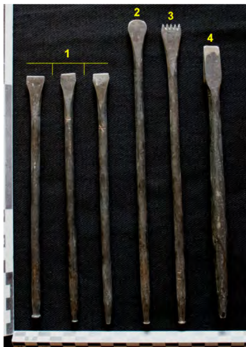
Figure 5. Various types of carving tools used in the process of making stone elements in Roman times: 1. flat chisels; 2. round chisel; 3. tooth chisel; 4. channeling chisel.
