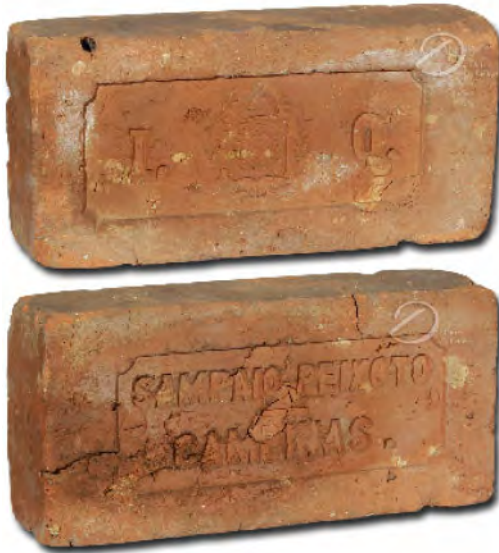
Figure 2. Brick produced at Sampaio Peixoto's Imperial Brick Factory. The name of the company and the imperial coat of arms are stamped on the brick. Dimensions: 26.2 cm × 7.3 cm × 12.9 cm. Source: Dutra auctions. Available at: http://www.dutraleiloes.com.br/2018/1139/catalogo2.asp . Accessed 26 November 2020.
