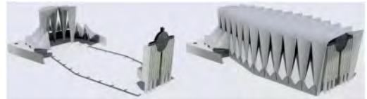
Figure 9. Church roof arrangement. Left show the radial disposition of pillars and hyperbolic paraboloid that cover the chancel and the façade structure. Right the disposition of the twelve elements that form the roof (Image Moisés Escárcega).
