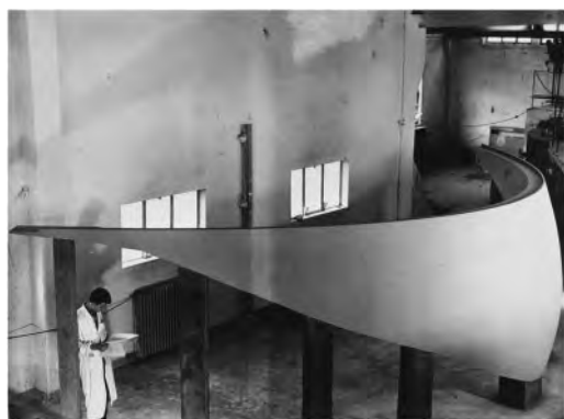
Figure 1. Valle di Lei dam on the Reno di Lei River, arch-gravity, double-curvature, preliminary model of wood at Ismes, scale 1:66, 1957 (SIXXIdata: Historical Archive of Ismes).
