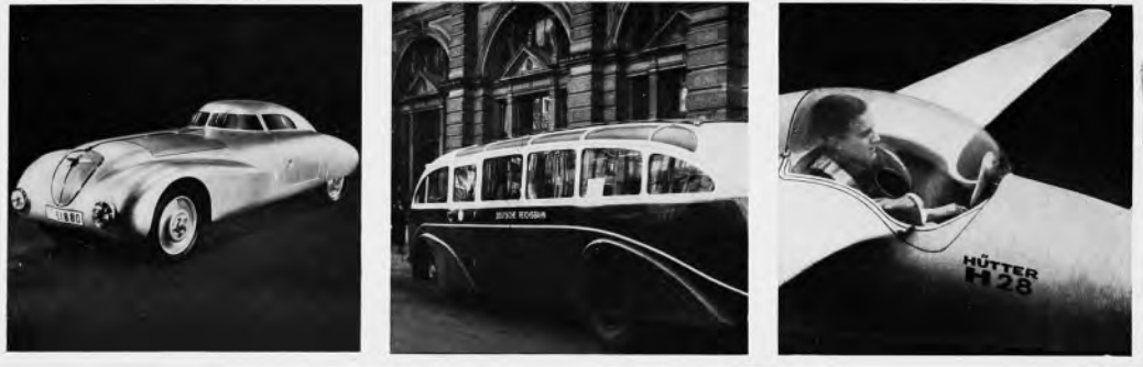
Figure 2. Examples of transparent Plexiglas windows in the 1930s by Röhm & Haas, applied to cars, buses and airplanes (Röhm & Haas A. G. 1936, 10).
