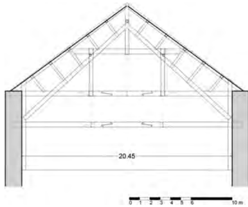
Figure 2. Cross section of the roof of the Opéra Royal in Versailles (Survey plan: author).
