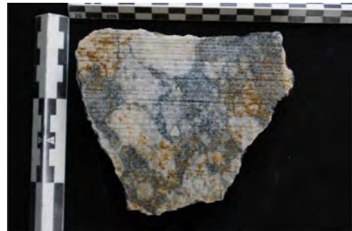
Figure 3. View of the back surface of a cladding ballast ( crusta ) covered by sawing traces. Note how, unlike the previous image, the grooves are more marked and separated from each other.
