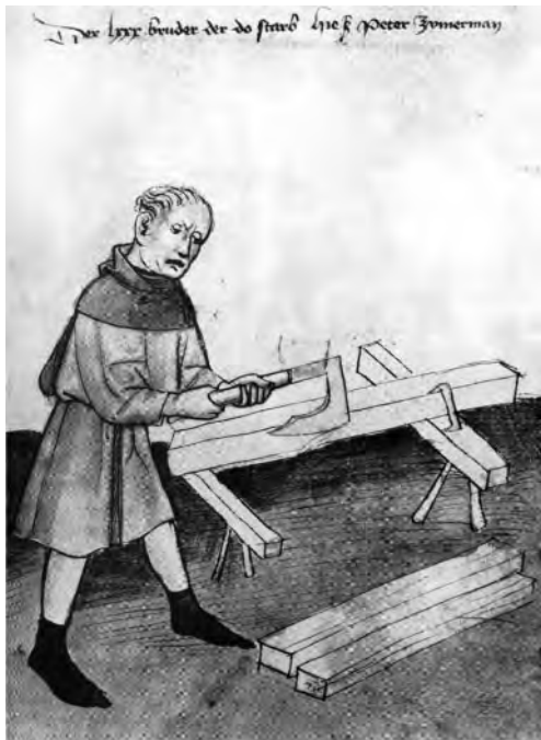
Figure 13. A carpenter smoothing pre-treated building material with a broad axe, 1425, cf. Schadwinkel & Heine 1986.
