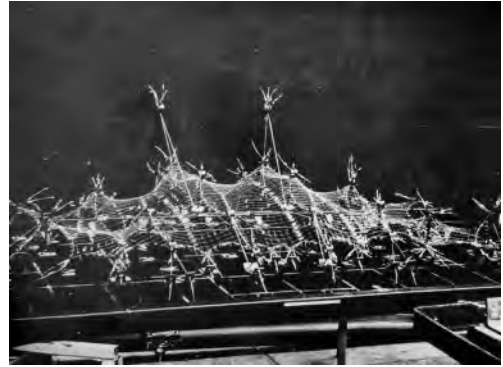
Figure 2. Measurement model of the sports hall at a scale of 1:125 (Bach 1975, 286).
