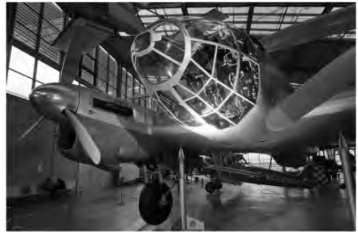
Figure 4. Front cockpit with gun outlet of the He 111 H16, a standard German Airforce bomber during World War II, built after 1937. DM München, Inv.-No. 79339 (Deutsches Museum, Munich, Archiv, CD64549).
