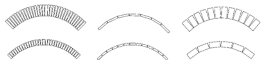
Figure 1. Main brick arrangements in a barrel vault: from left to right, radial brick, tile vault and vault by slices (Rabasa 2020).
