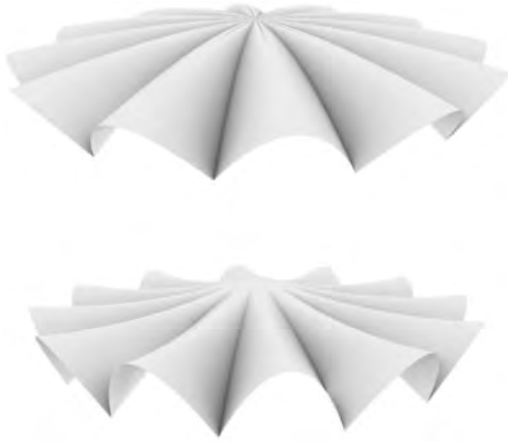
Figure 11. 3D shells modeling. Top: José Hernández Casas's design. Bottom: Felix Candela's design.
