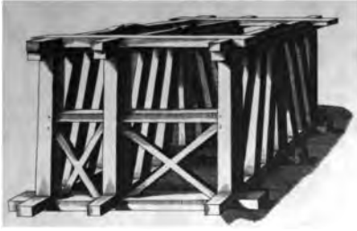
Figure 9. Box construction with numerous braces in the truss.
