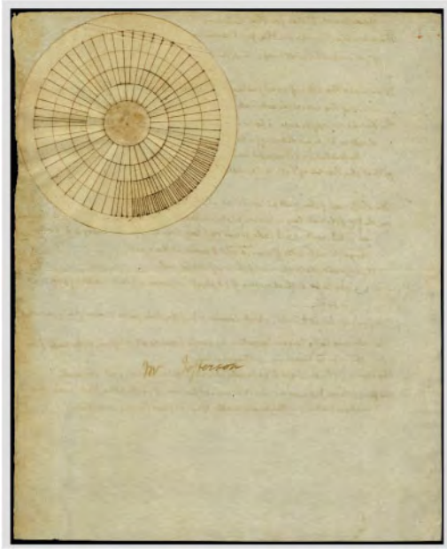
Figure 6. Delorme framing plan for the Rotunda at the University of Virginia drawn when Jefferson was in his upper 70s. The density of linework in the lower right corner of the image is indicative of the sub-ribs required on lower levels of the dome.
