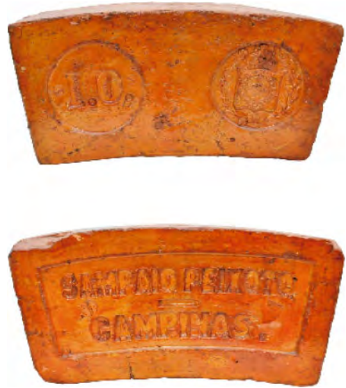
Figure 4. Brick produced at Sampaio Peixoto's Imperial Brick Factory. Product has a particular shape to be used for the construction of arches. The name of the company and the imperial coat of arms are stamped on the brick. Source: Miguel Sales auction and Art Space. Available at https://www.miguelsalles.com.br/peca.asp?ID=5168169 . Accessed 26 November 2020.
