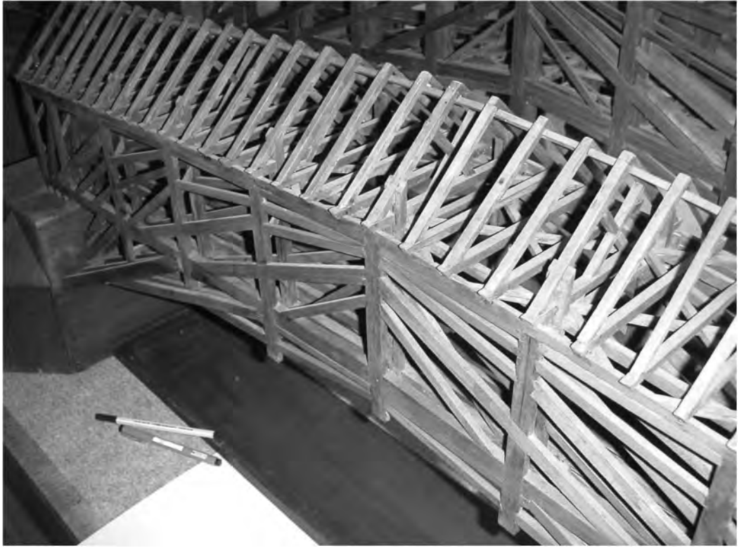
Figure 3. Model of the largest span which stood from 1767 to 1813, Town Museum Meissen, Inv. No. 331 (Photo: author).
