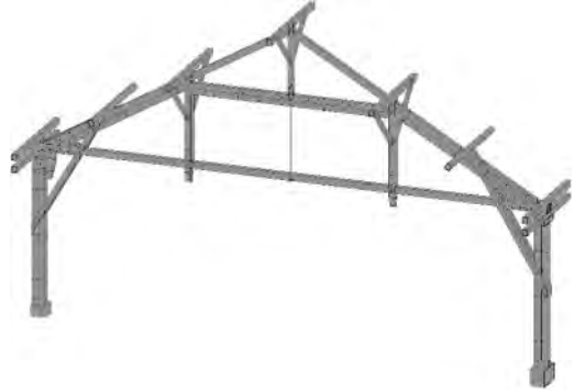
Figure 2. Principal truss of the riding hall in Frauenfeld, built 1863, span 17.1 m (Tobias Lenggenhager 2019).
