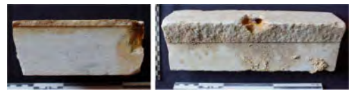
Figure 4. Examples of large-format marble decorative cornices on the back side of which the distal end breakage caused by saw cutting is observed.
