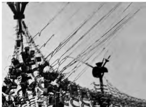
Figure 6. Test setup for simulating the uplift due to the wind (Bach 1975, 291).
