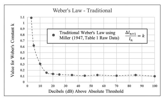
FIGURE 1.1 Traditional Form of Weber's Law Demonstrating the Nonconstant Error Near Absolute Threshold Using Miller (1947) Raw Acoustic Data.
